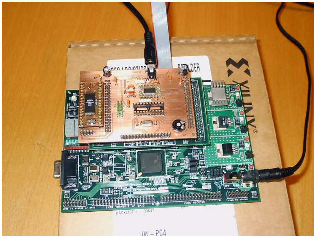
Fig. 8. Xilinx devel board, DAC board
